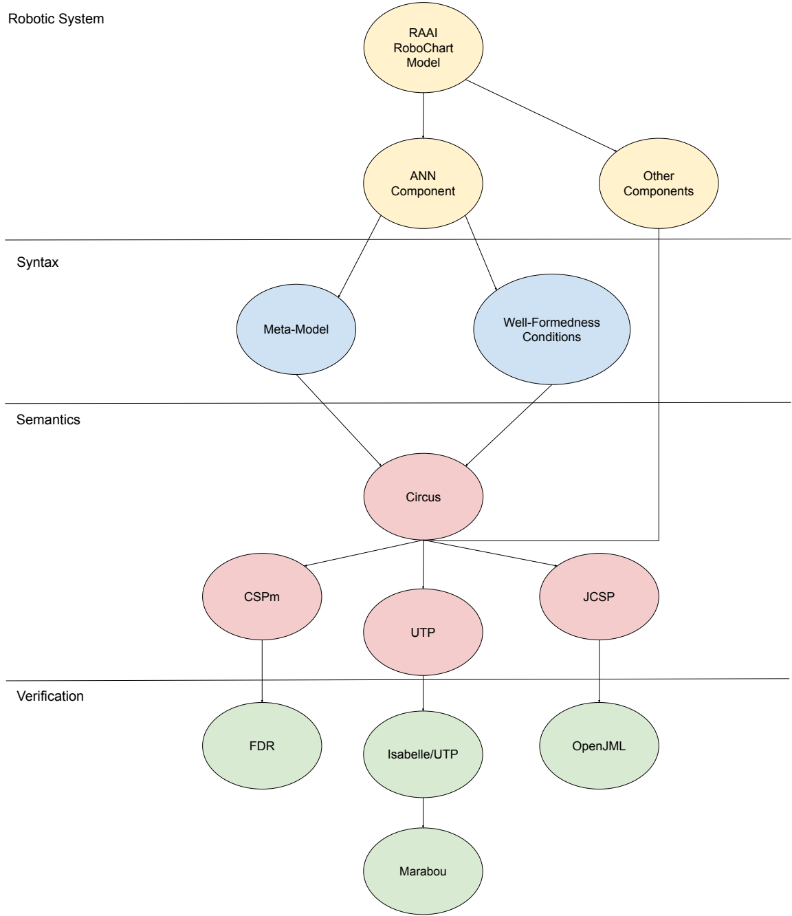
Figure 3.3: The structure of our verification framework: the nodes in Robotic System represent the broad structure of a RoboChart model with an ANN component; the nodes in Syntax represent the artefacts we have developed to support modelling of ANN components; the nodes in Semantics represent semantic models of ANN components, and their implementations; finally, the nodes in Verification represent verification tools and frameworks.
